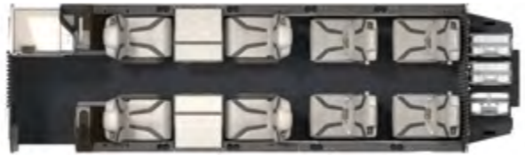
Executive 4 + 4 Seat Interior Whenever the need arises, the pilot can simply add or remove the four quick-release, lightweight commuter seats, allowing flexible accommodation for four to eight passengers.
