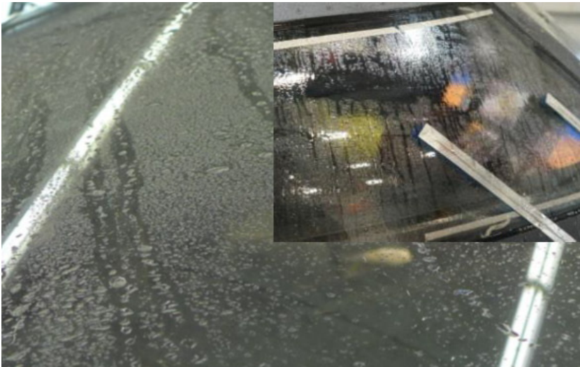
Figure 2-7-3: Windshields - Rain repellent (unsatisfactory condition)
