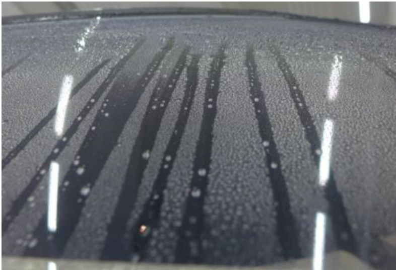
Figure 2-7-1: Windshields - Rain repellent (good condition)
