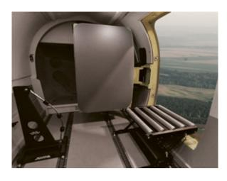
An optional integrated utility and jump door increases the number of roles while retaining the standard cargo door functionality
