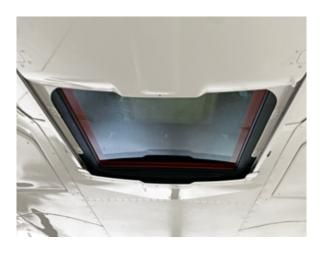
The two hatches ( $21 \times 21$  and  $21 \times 9$  inches/ $53 \times 53$  and  $53 \times 23$  centimetres) can be opened in flight enabling scanning and photography
