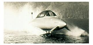
**1974** Manufacture of the two-seat ZISCH 74 boat with a 265 hp 4-disc rotary-cylinder engine on behalf of Dr. Wankel. Successful trial run on Lake Lucerne in the summer of 1975. Experiment was not pursued further.
