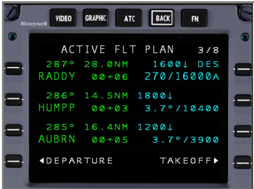
Figure 5. (Sheet 1 of 1) Old Constraint is Incorrectly Retained After Activating the Amended FPLN
